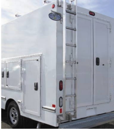
Shown with optional aluminum ladder rack and removable access ladder
